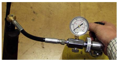
hose, if you do not vent the hose you will not be able to remove the female from the rifle). Now the female connector can be removed from the rifle and end cap (S483) can be replaced over the male connector ensuring not to over-tighten.
