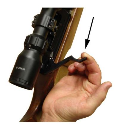
Note! It is very important that the cocking lever is pulled back to the correct position. In one positive motion. The magazine indexes to the next pellet position as the bolt is retracted and it is possible for a partial index if the lever is not pulled back fully.
